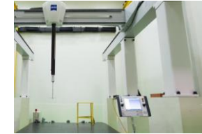
CMM Co-ordinate Measuring Machine with least count of 0.1 Microns and volumetric accuracy of 7 Microns. Largest Test Facility in Asia
