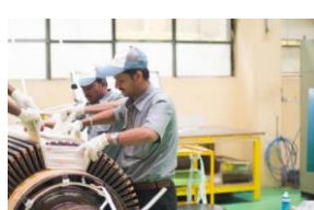
Cylindrical Rotor Winding Coil insertion and winding
