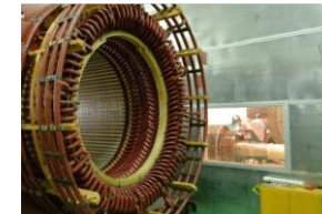
Electrical Testing Chamber High voltage and partial discharge tests to ensure longevity
