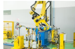
Tapping Machine Completely robotic with six axis and tapes also the overhang portion
