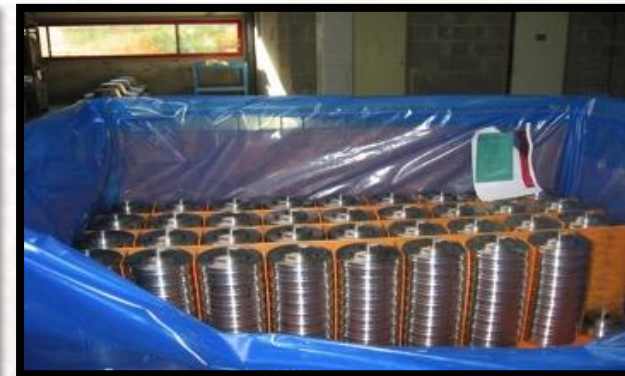
Application for Anti-Corrosive VCI Material
