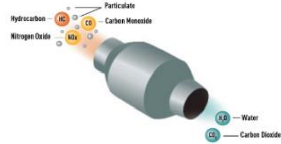
DIESEL OXIDATION CATALYST- DOC
