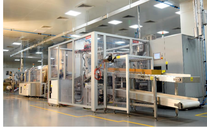
300 UPM Fully Automatic with Robotic pick up Tube Packing Line from Norden
