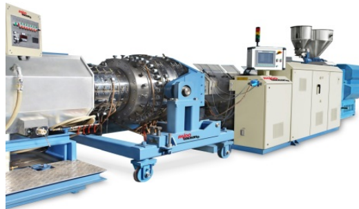
FLOW E X - Twin Screw PVC Pipe Plant
