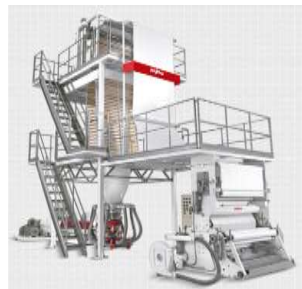
FOMEX™ - PS/PE Foam Extrusion Lines
