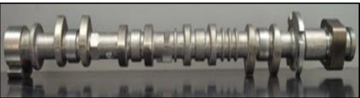
Hybrid Camshaft – Chilled Casting + Steel Fuel Lobe
