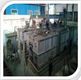
Spherodizing & Annealing Machines
