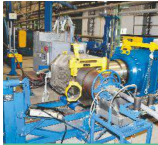
Lead Sheathing Line
