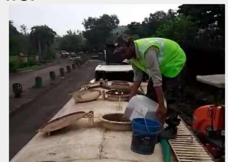
Addition of Liquid Chemical Additive
