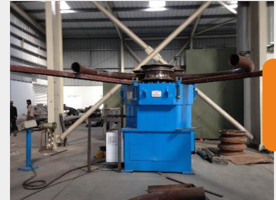
Pipe Rolling Machine pto Ø200 X 8 Mm
