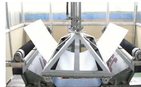
Withstood > 180 Mpa (Standard 90 Mpa as per EN 12150-1)
