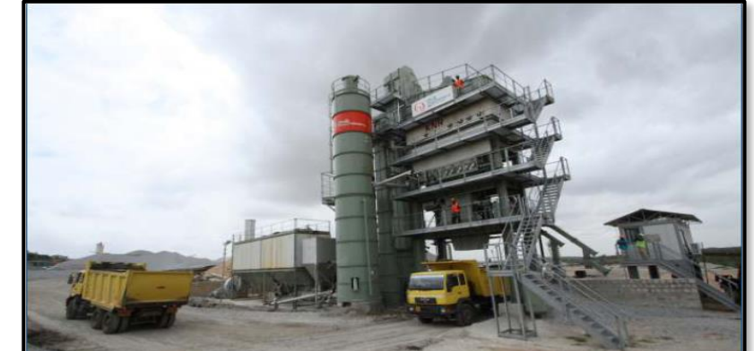
240 TPH D & G Hot Mix Plant
