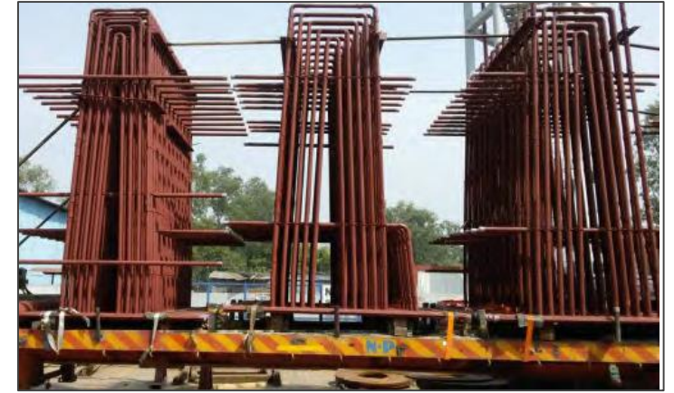
Membrane Panel with Evaporator Coil Assembly
