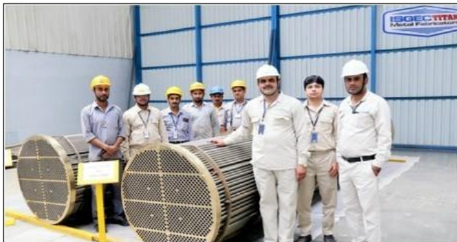
Titanium Tube Bundles for a Refinery
