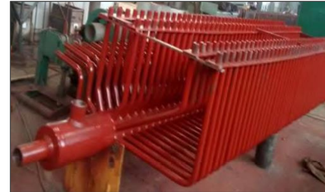
Primary Super Heater Header
