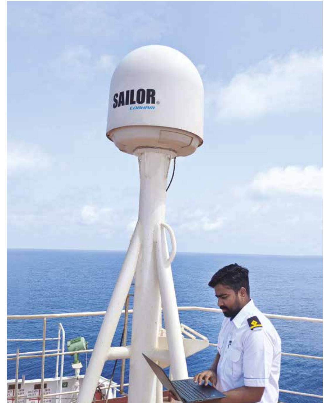
Satellite communication through a Very-Small-Aperture-Terminal (VSAT) on a moving ship is used for high-speed connectivity at sea.
