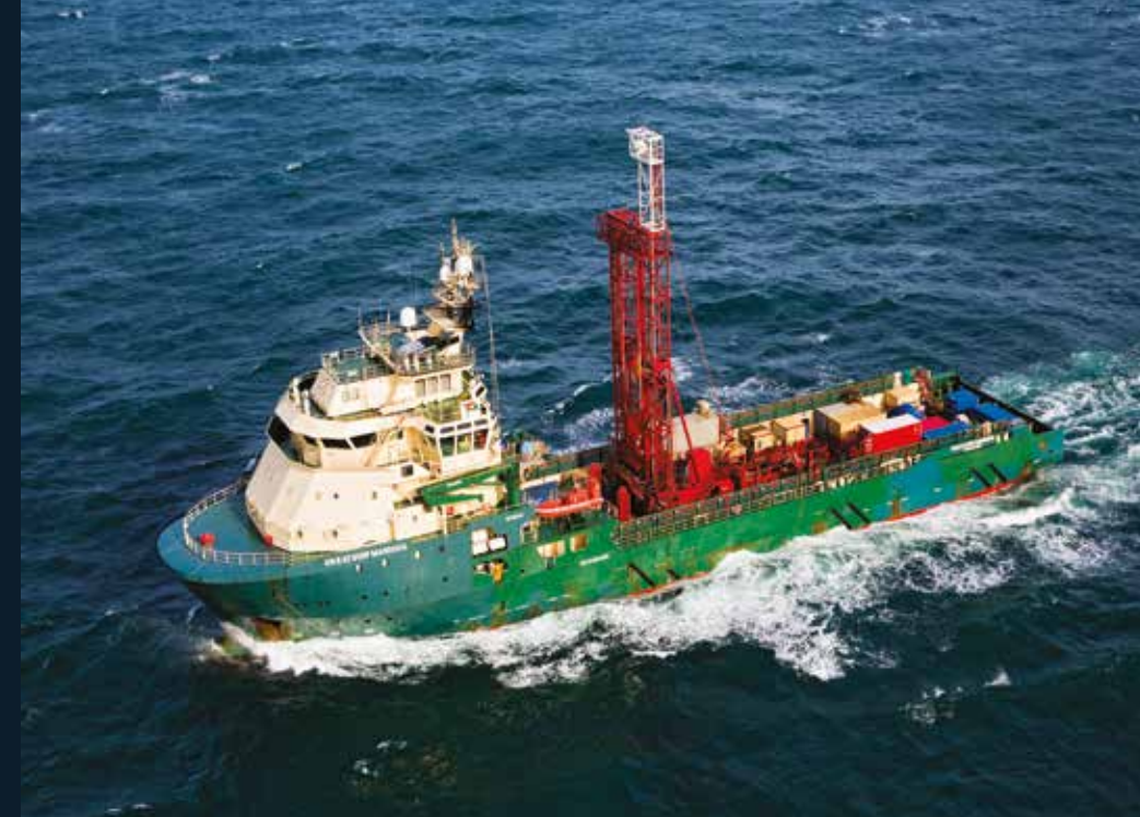
Greatship Manisha is a DP II, 4,221 dwt diesel-electric MPSSV built at Keppel Singmarine.
