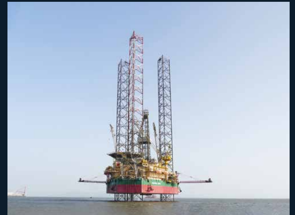
Greatdrill Chitra , a 350-ft water depth, independent leg cantilever jack-up rig. She is capable of drilling wells to depth of 30,000 ft.
