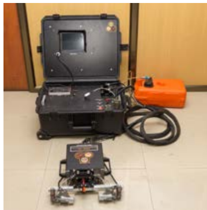
Artificial Intelligence (AI) enabled weld inspection tool using advanced phased array technique to replace manual radiography (AI-UT)
