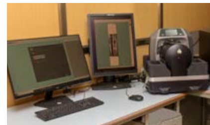
Artificial Intelligence (AI) enabled weld inspection tool with computerized radiography (AI-RT)
