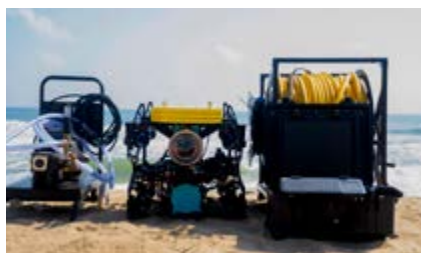
Artificial Intelligence (AI) enabled remotely operated vehicle (AI-ROV) for under water inspections
