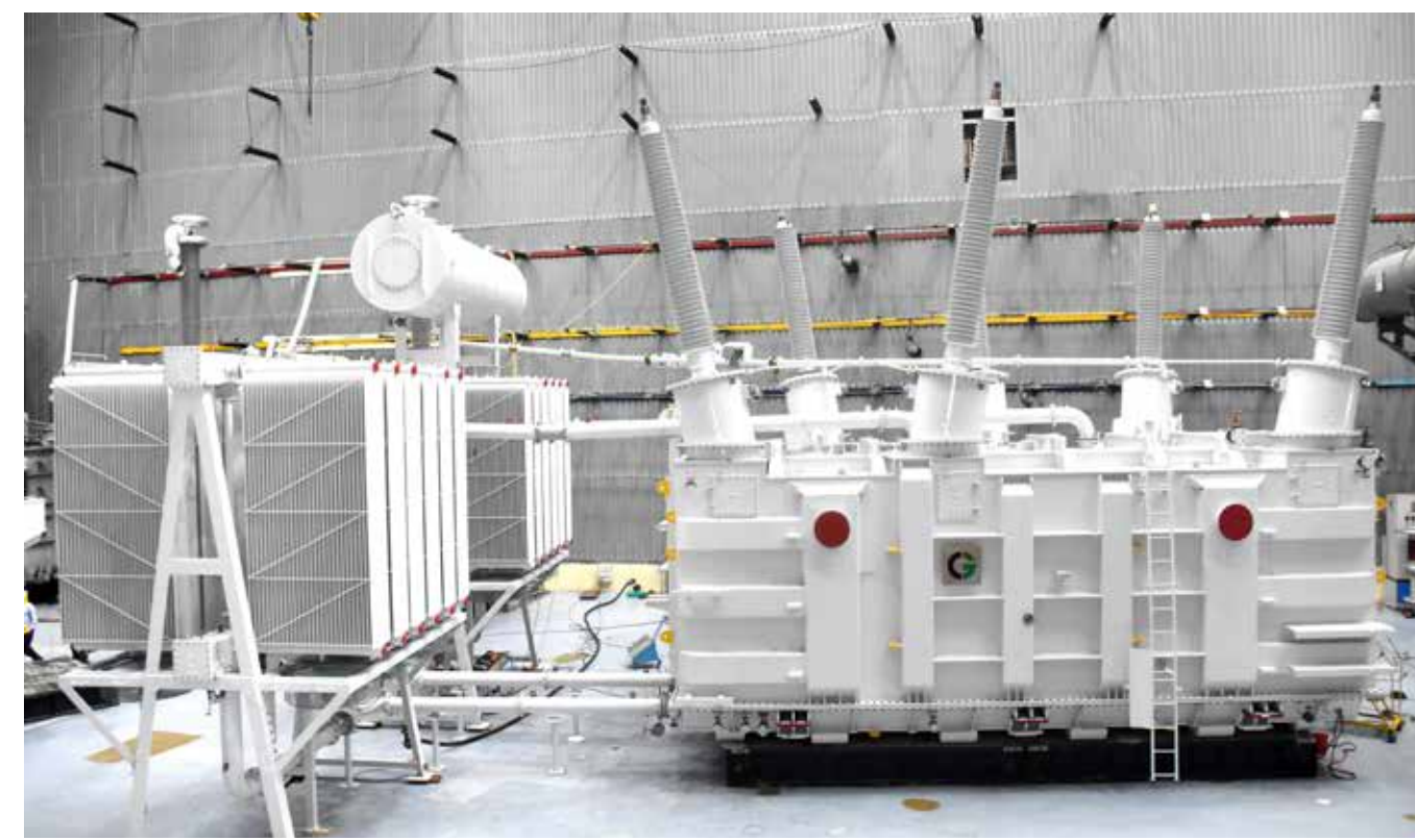
500MVA, 420KV AUTO-TRANSFORMER
