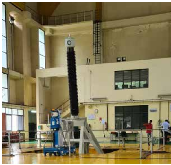
S1-420 kV Bushing under Seismic Test at 0.5g at CPRI
