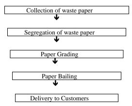
The Company deals in procurement of waste paper from waste paper sellers and segregates the collected waste paper into different grades based on the quality of waste paper procured by it. After grading the waste paper, the same is baled and stored in the godown. Based on the orders placed by the paper mills, the required quantity of graded paper bales, are dispatched and payment is received as per the agreed payment terms.
