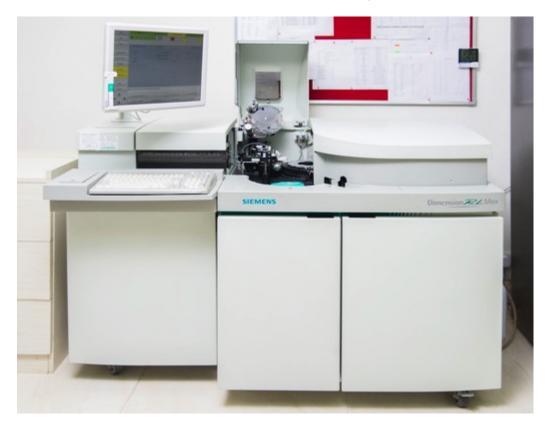
Mode: Fully automaticBiochemistry machine with Random Access Throughput: 400 tests/hour with 60 samples processed in one Go
