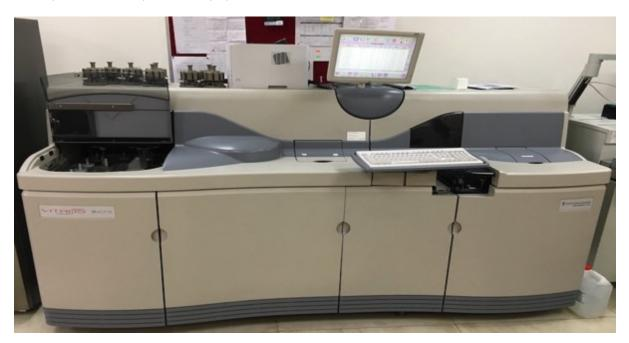
Mode: Fully automaticBiochemistry machine with Random Access Throughput: 700 tests/hour with 160 samples processed in one Go
