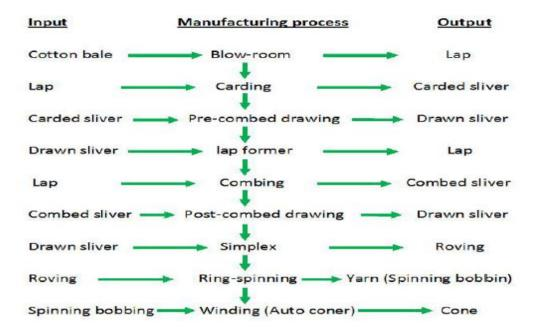
**Blow room:** This is the first process of cleaning the cotton. The raw cotton pressed in to the bales is in very compact form and contains a lot of agro impurities and foreign particles. In this process the cotton is opened up for further cleaning. There is homogeneous mixing of cotton. The opening itself liberates some heavy impurities which is sucked away in to waste collection bags. Cotton is further cleaned by beating and saw tooth type combing points
