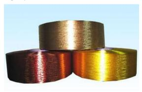
The fibers and filaments are fully impregnated with pigment since adding master batch colorant at the beginning. Dope dyed yarn is an energy saving & environmental friendly product. Due to dope dyed yarns are created by adding masterbatch colorant to the polymer melt in spinning, it substituted the most polluting process of dyeing.
