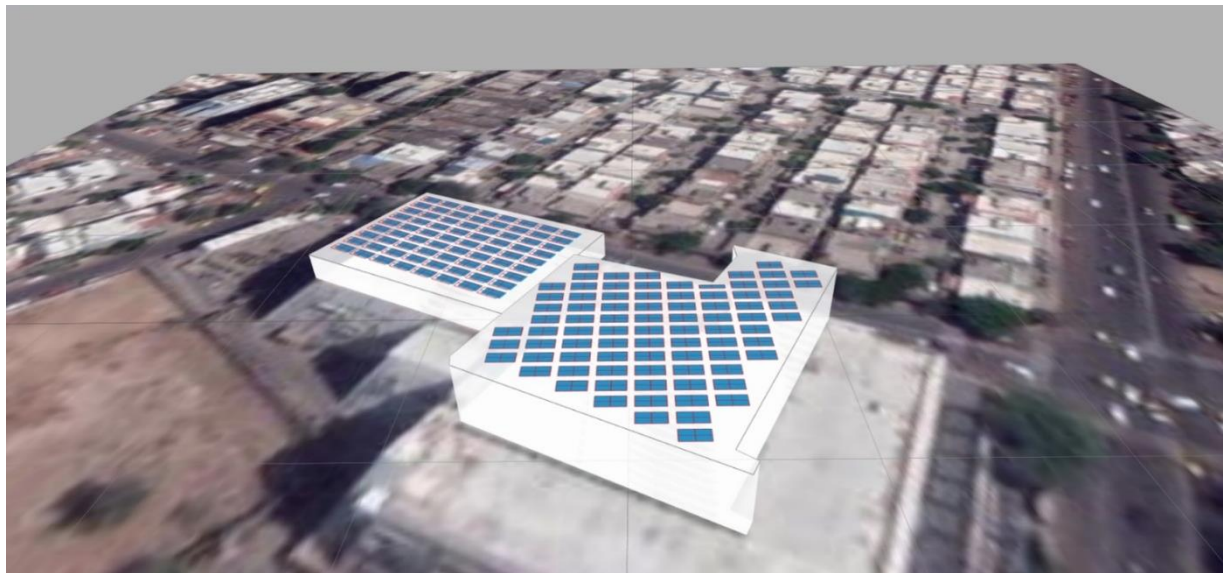
Image: Simulation result of Solar Panels on the roof designed on Sun Analyzer
