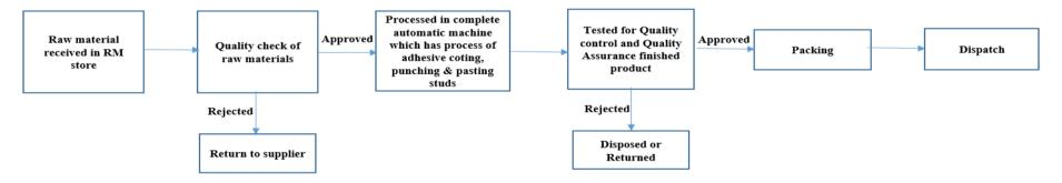
ECG Electrode is used for conducting an electrocardiogram. The ECG Electrode is manufactured on an automated machine. The Medical Grade Adhesive Roll is fed on an automated ECG Machine which cut the Adhesive roll into small round pieces. The Electrode for taking ECG is fed into a vibratory bowl and is fixed on medical-grade Tape and each Electrode is glued by the machine and then the Electrodes are pressed into Tape by automatic ECG Machine then they are packed into an aluminum pouch.
