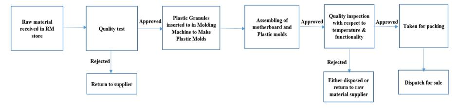
Digital Thermometer is used for Checking body temperature The Thermometer consists of plastic parts, a PCB, and a sensor The Plastic parts are first moulded on injection moulding machines, PCB and Sensor are welded and inserted into the Plastic body. After inserting PCB and sensor the same is checked by testing instrument and they quality passed instrument are packed for dispatch.
