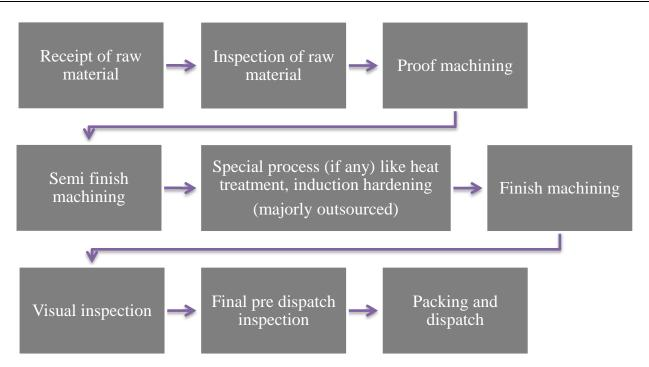
The process undergone in the manufacturing of precision machined components is briefly described hereunder:
