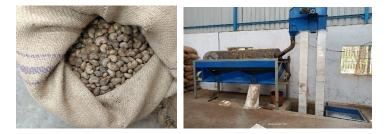
The first processing operation is the removal of foreign matter and dirt from the nuts. Processing Raw Cashew Nuts into Dust Cleaner to remove Foreign Matters and Dirt and taking the material directly to Tank for Boiling.
