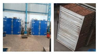
Separated Nuts collected from Scooping Line are filling in Tray and Trolley and loaded in Dryer to remove Oil from Husk of the cashew. Drying process vary between 350 Minutes to 480 Minutes depending on the Raw Material.
