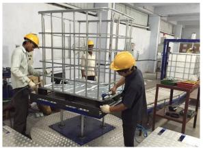
Manufacturing of cage for rigid Intermediate Bulk Containers
