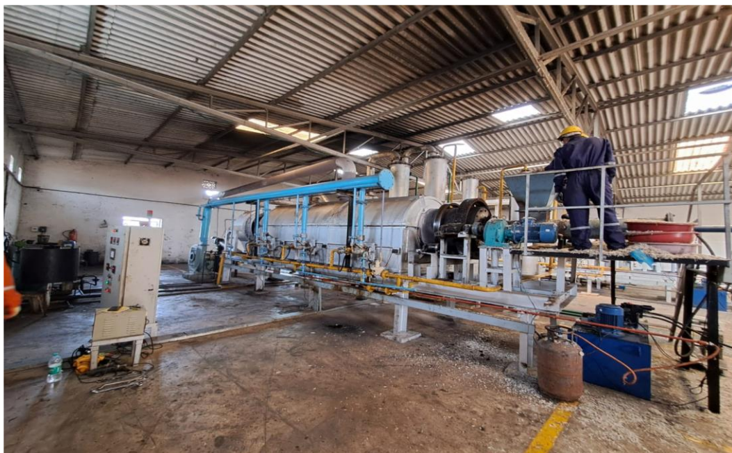
Workers Putting the Plastic waste in the machine to process it and convert it into Oil by the process of Pyrolysis
