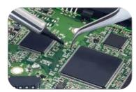
PCB assembly is the process of connecting electronic components onto PCBs. Components are placed onto the foot prints or inserted into the via holes and soldered to complete the electronic circuitry.
