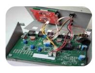
Also known as systems integration, box builds can be anything from a simple PCBA housed in a small enclosure, to a cabinet housing a complex electromechanical system. The box build process involves enclosure fabrication, assembling the various PCBAs and cables harness assemblies, installation of sub-assemblies and components and routing of cabling or wire harnesses.
