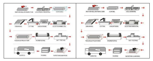
The manufacturing process for seamless tubes and pipes is a well calibrated process in line with applicable industry standards in India. A brief description of the step-by-step manufacturing process (for both the methods as indicated above) is provided below:
