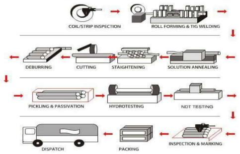
The manufacturing process for Welded Tubes and Pipes is a well calibrated process in line with applicable industry standards in India. A brief description of the step-by-step manufacturing process (as indicated above) is provided below:
