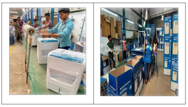
We have total 3 Conveyor Assembly Line for fast production 2 Assembly Line for Air Cooler and 1 Assembly Line for Electric Geysers, which can be increase depending upon the requirement.
