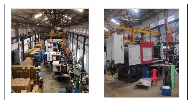
We have Moulding Unit Setup under same roof with 8 Moulding Machines- 3 of 100 Tons, 1 of 170 Tons, 1 of 280 Tons, 1 of 350 Tons, 1 of 450 Tons and 1 of 775 Tons.
