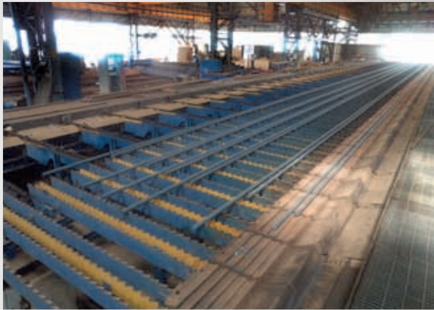
An overview of cooling bed of newly erected Rolling Mill.
