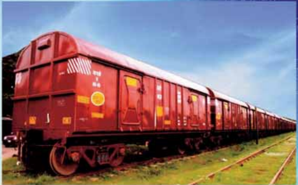
Broad Gauge Bogie Covered Wagon (BCNHL) with Sliding Door, made of High Tensile Micro Alloy Steel.
