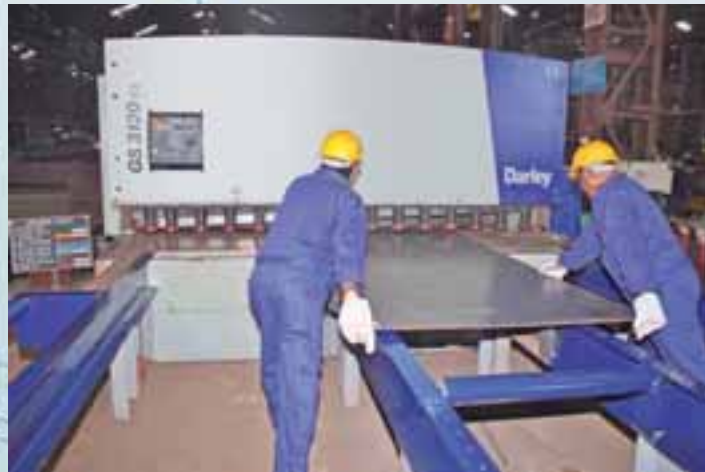
CNC Shearing -Make-Darley,Holland
