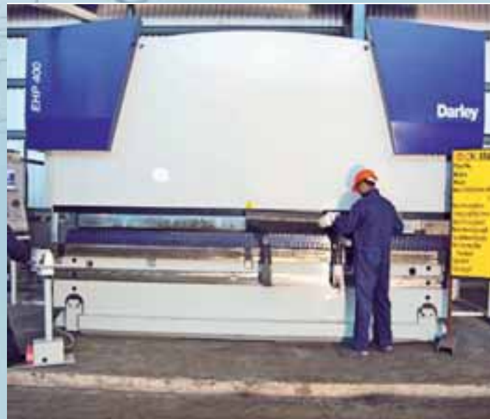
CNC Brake Press (400T)-Make-Darley,Holland
