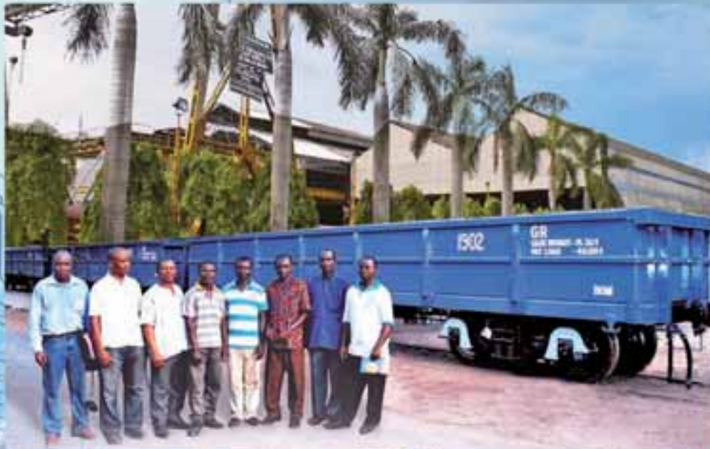
Meter Gauge Bogie Open Mineral Wagon (‘BOMW’) for Republic of Ghana, with their team.
