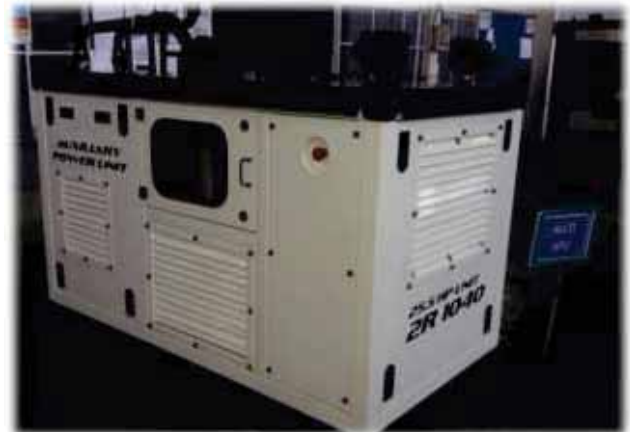
Railways Auxiliary Power unit
