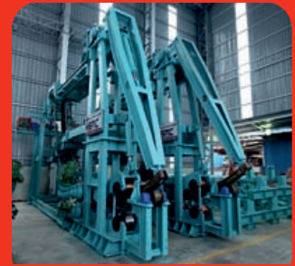
Continuous Casting Machine
