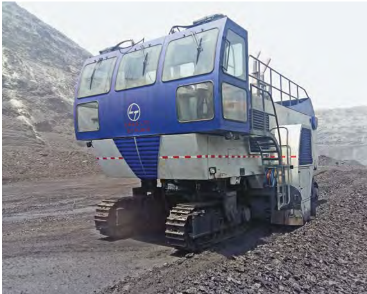
L&T's KSM-404, the largest surface miner in Indian coal mine at Gevra, Chhattisgarh
