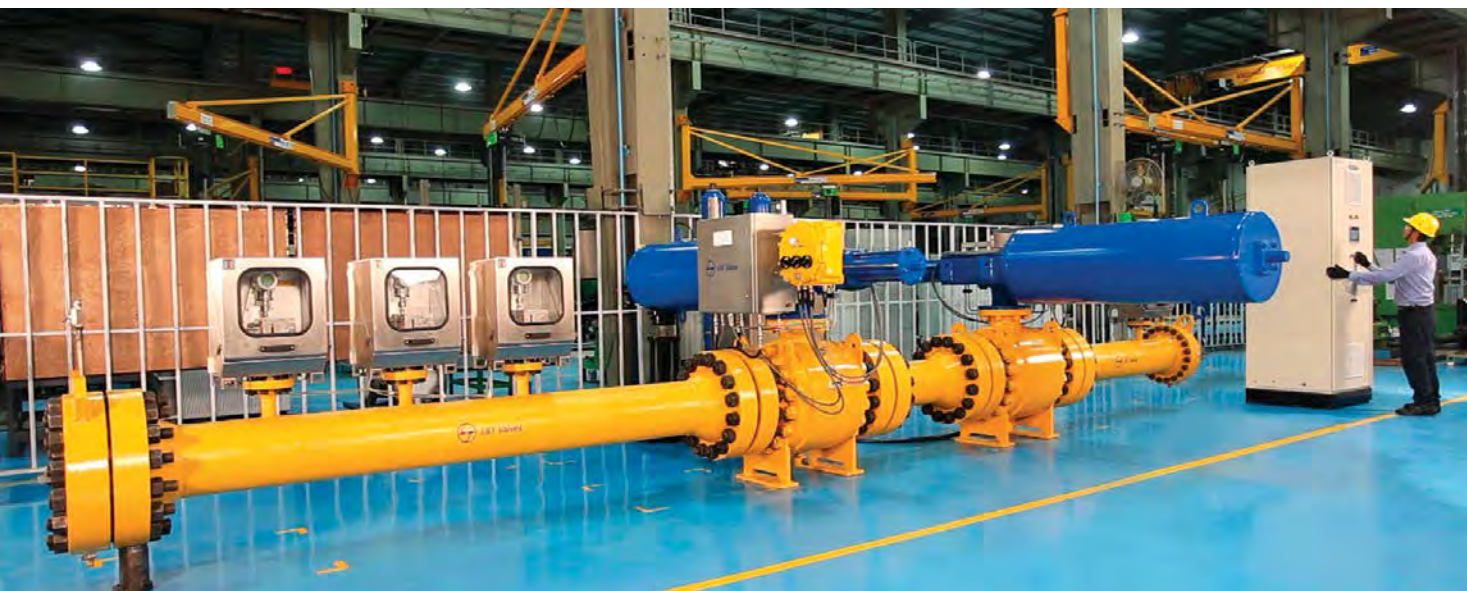
The first HIPPS (High Integrity Pressure Protection System) designed and manufactured in India.
