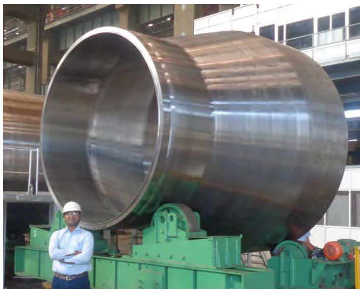
Nuclear Steam Generator Cone Shell - 16 MT
