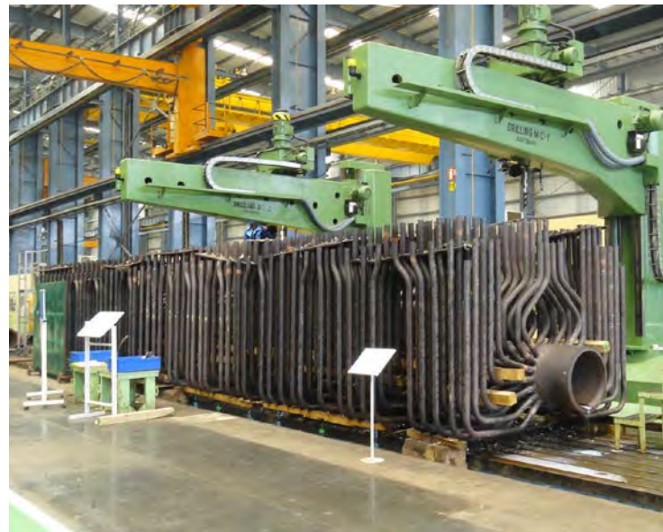
Boiler internals being manufactured at Hazira, Gujarat
