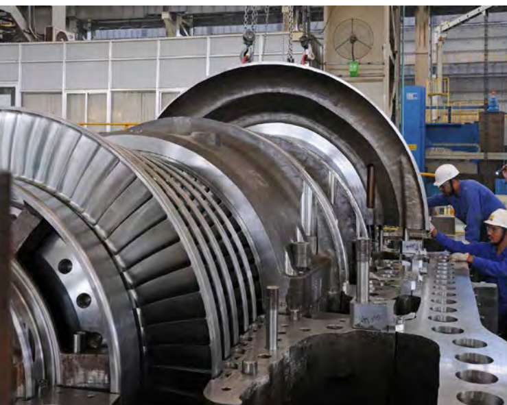
Supercritical turbine being manufactured at Hazira, Gujarat
