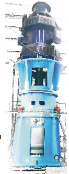
Primary Heat transfer pump for the 500 MW Prototype Fast Breeder Reactor (PFBR) at Kalpakkam, Tamil Nadu
