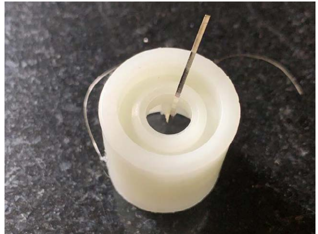
During COVID-19 crisis, MIDHANI has developed and supplied Nickel Wire (0.16 mm) with purity ~100% which was critically required for the manufacture of Oxygen sensor pertaining to the "Critical Core Ventilator"
