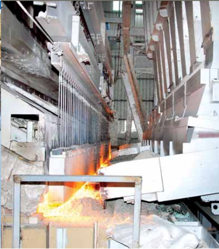
Batch being fed into the furnace
