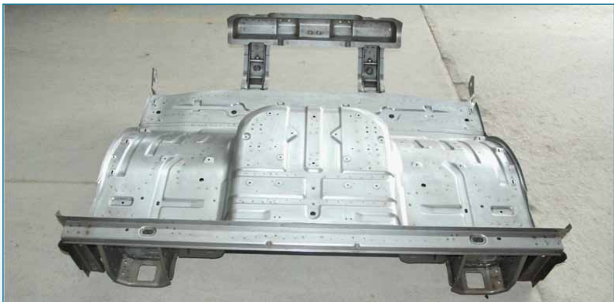
Cabin Floor Structure
