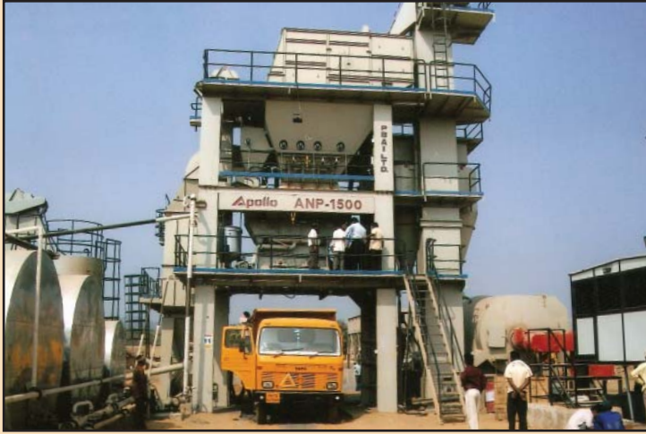
124 TPH ASPHALT BATCHMIX PLANT INSTALLED AT SAWANTWADI
