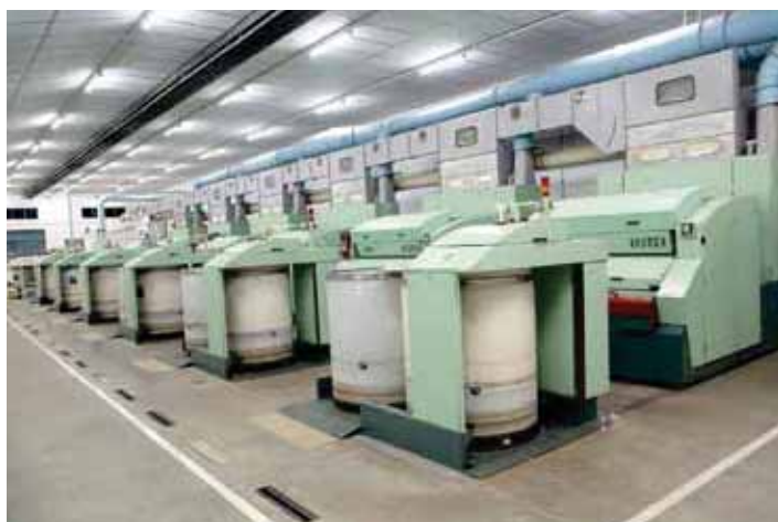
A view of Rieter C60 Carding Machines installed at our unit Rajapalaiyam Spintext.
