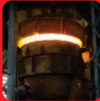
Electrotherm Refining Furnace
