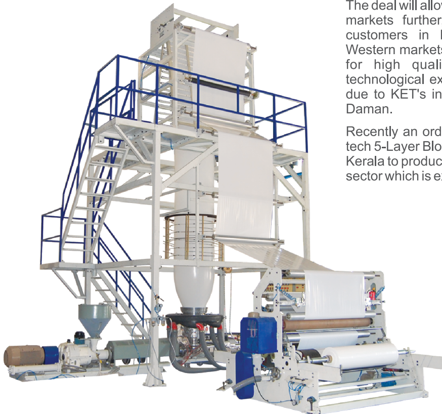
Multi Layer Blown Film Plant
