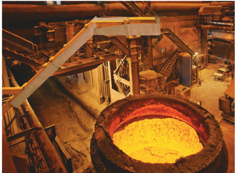
▲ Ladle Laser Scanner
