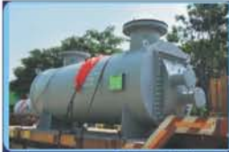
Compressor Inter Coolers
