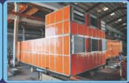
Air Handling Units
