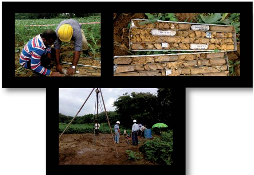
Fig-13: Geotechnical Drilling and logging, Ganajur Main Prospect
