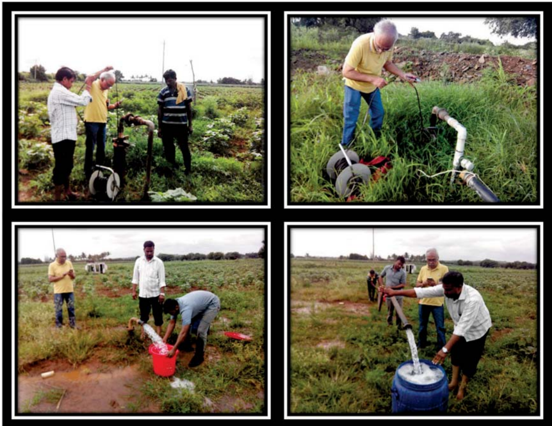
Fig-14: Hydrogeological consultant carrying out ground water tests
