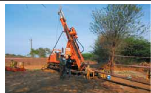
Fig-8 : Diamond Core Drilling operation at Ganajur Main Prospect, Ganajur-Karajgi PL.
