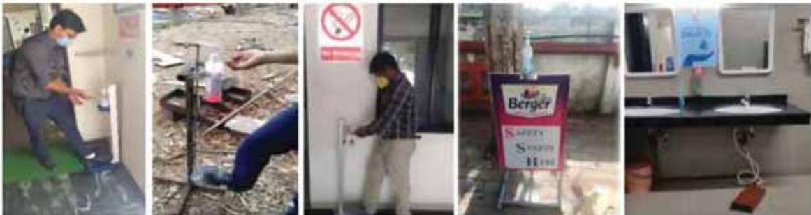
In-house fabricated foot operated sanitizer dispenser, wash basins & motion sensor taps
