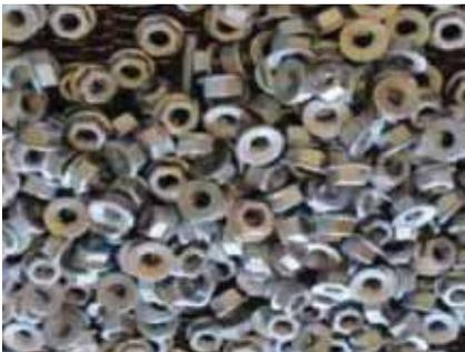
Zinc flake anticorrosive coating for fasteners
