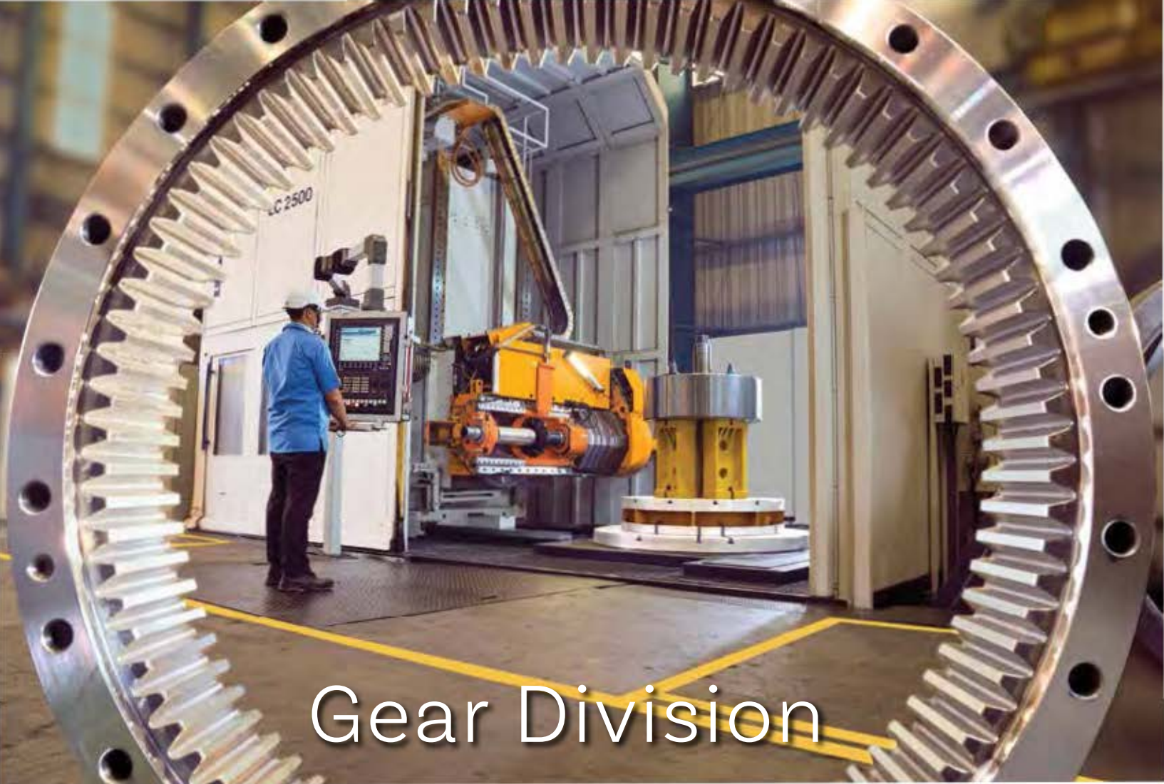
▲ LIEBHERR LC2500 - CNC Gear Hobbing machine - 3000 mm Dia
