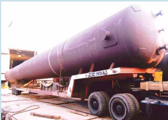
200 M3 Oxygen Buffer Vessel (3.7m dia, 21m long, 82T weight)
